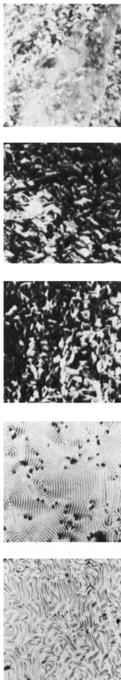
FIGURE 3 Photomicrographs (64x), taken with crossed polars, of the induced cholesteric phase of PAA/TMAB for chiral weight fractions (left to right): (a) 0.026, (b) 0.057, (c) 0.097, (d) 0.333 and (e) 0.745.
